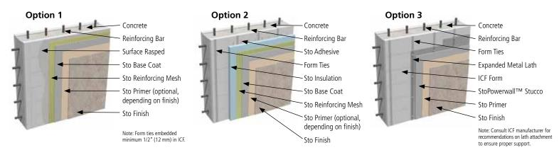
Option 1: Coating System Recommended when the walls are straight and flat with little leveling needed and ties are embedded at least 1/2 inch inside the ICF form.
